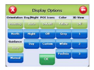
Orientation: Orients the Map screen so that the driving direction is heading up or North is always up
